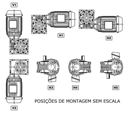
POSIÇÕES DE MONTAGEM SEM ESCALA
